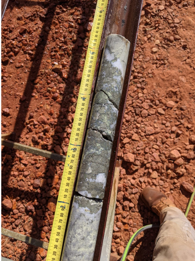
Photo 4 - Example of semi-massive pyrite/chalcopyrite ~ 347m in ETG0243
