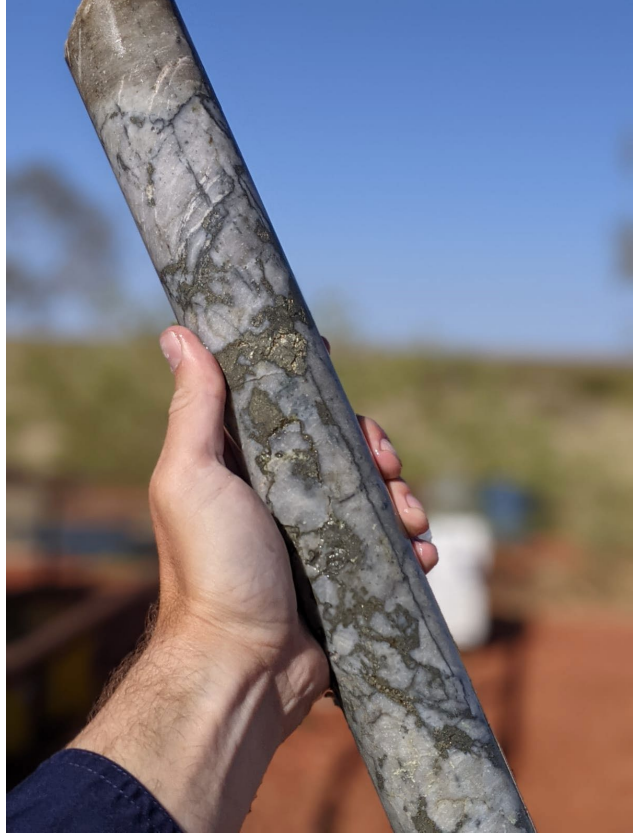
Photo 5 - Example of brecciated quartzite containing pyrite with fine chalcopyrite ~ 519m in ETG0243
