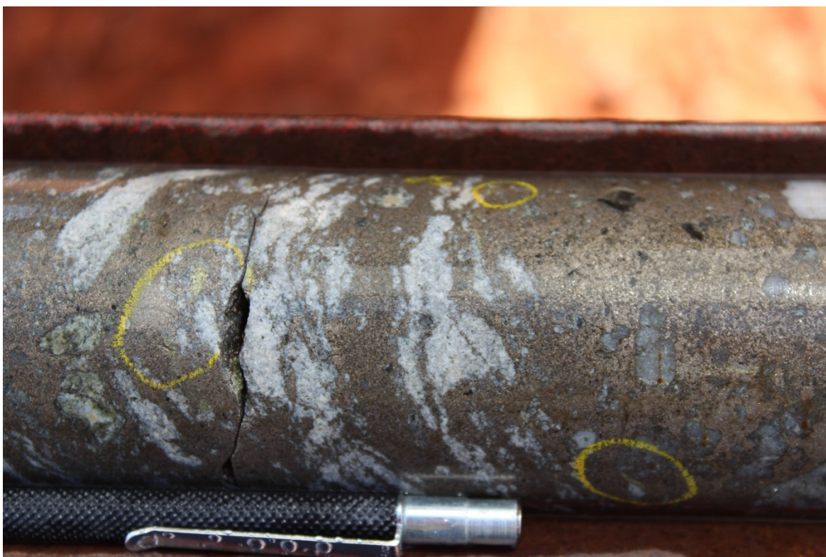
Photos 8. Example of semi-massive pyrrhotite with blebs of chalcopyrite at ~334m in ETG0241
